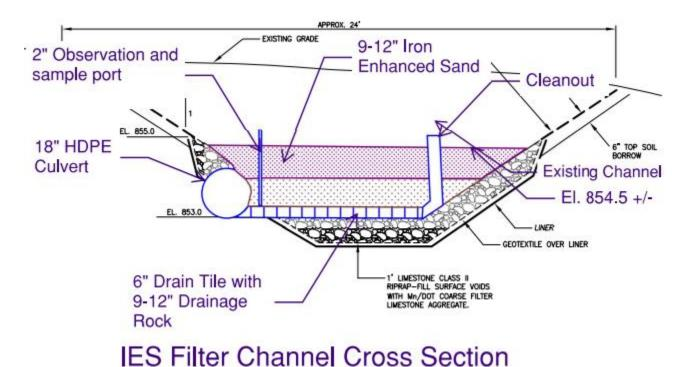
Figure 4. Typical cross section of the IES filter channel. Wenck Associates, Inc.
