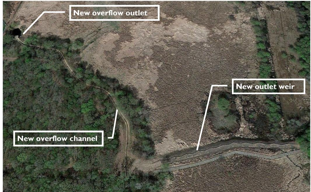
This 2011 project constructed a new outlet for a large flow-through wetland just upstream of Upper Twin Lake. This wetland has been found to be a significant source of nutrients to Upper Twin Lake - monitoring at the inlet and outlet found that phosphorus concentrations double as stormwater runoff flows through the wetland.
