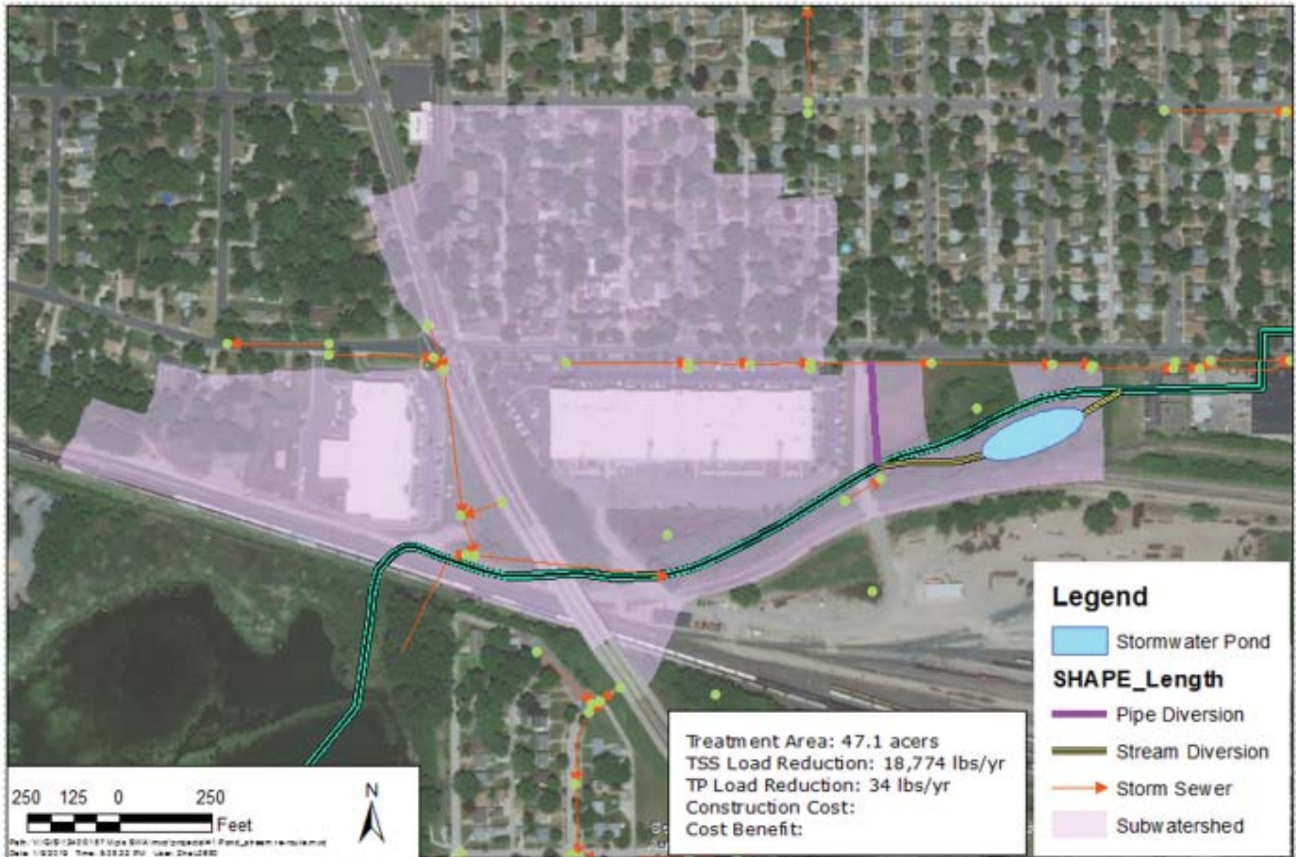
Figure 4-2 Project #1 Pond/stream re-route
