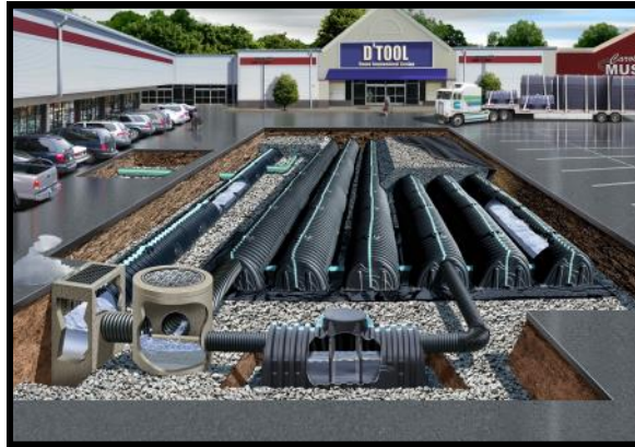
A cut view of an underground infiltration system. This system may be placed under a parking lot, park or other area to accommodate storage and infiltration of runoff.
