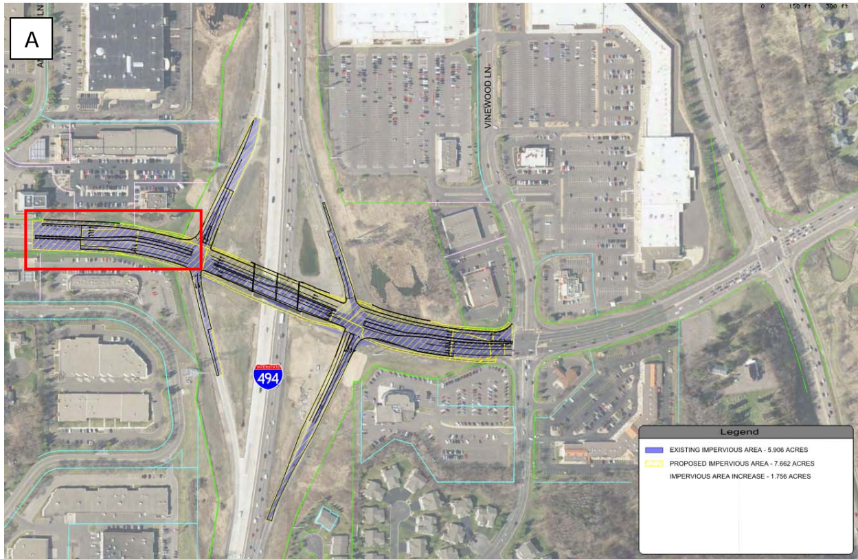
Figure 3. Increase in impervious in whole project area (A) and in Shingle Creek portion (B).
