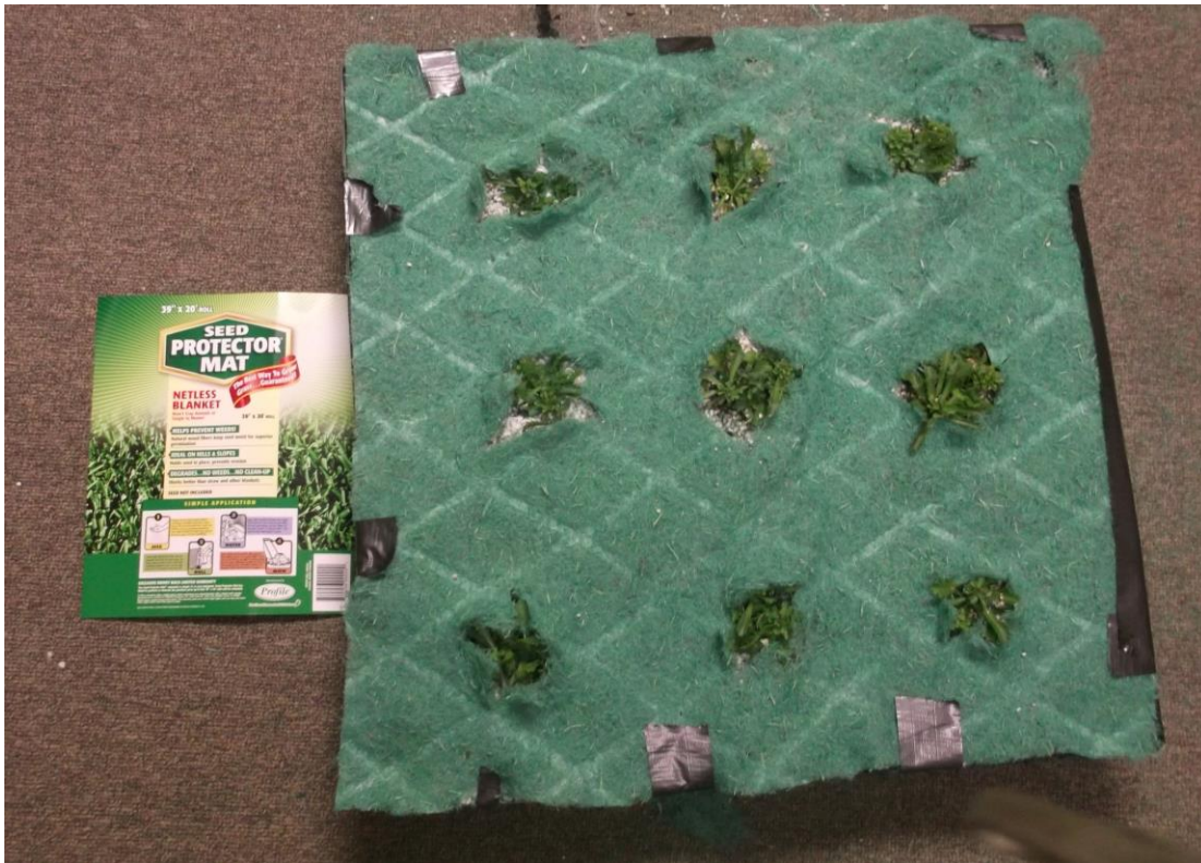
Figure 3.2. Erosion control fabric protecting the light-weight planting mix.
