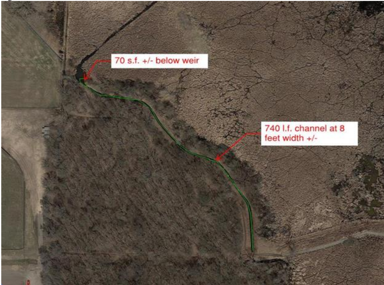
Figure 1. The overflow weir and channel at wetland 639W.
