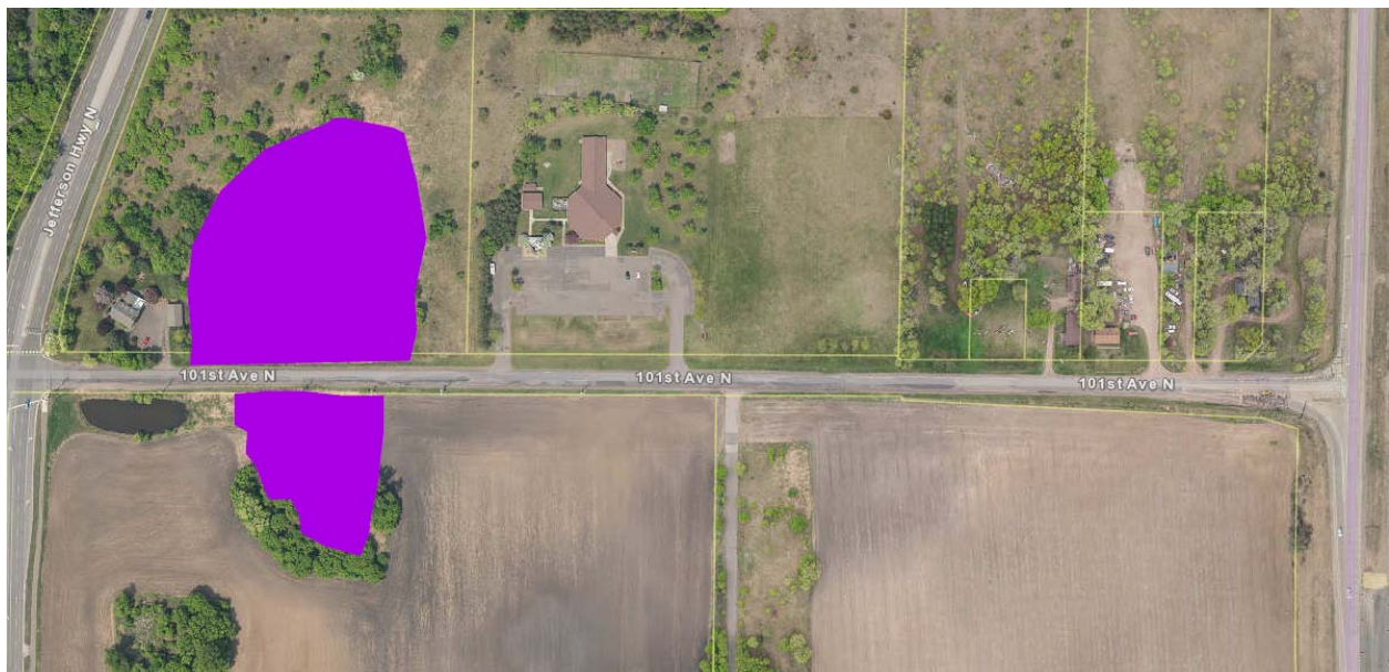
Figure 4. The DNR public water wetland on site. This wetland will have less than 20 feet of buffer on the sides adjacent to 101 st Ave because creating 20 feet of buffer would necessitate filling the wetland. However, all stormwater runoff from 101 st Ave and associated sidewalks/trails will be directed away from the wetland.
